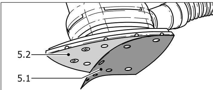
Simply press the abrasive (5.1) onto the sanding pad (5.2) and pull it off again after use.
